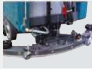
Curved steel squeegee, no stains or waste water residues after suction
